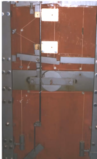
Figure 86. Modern safes have sensors that detect attacks and will lock themselves down.
