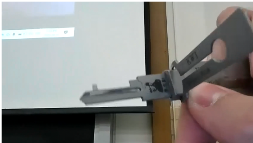
Figure 79. Slightly more modern picking tool which simulates a key as well as gives offsets for the notches
