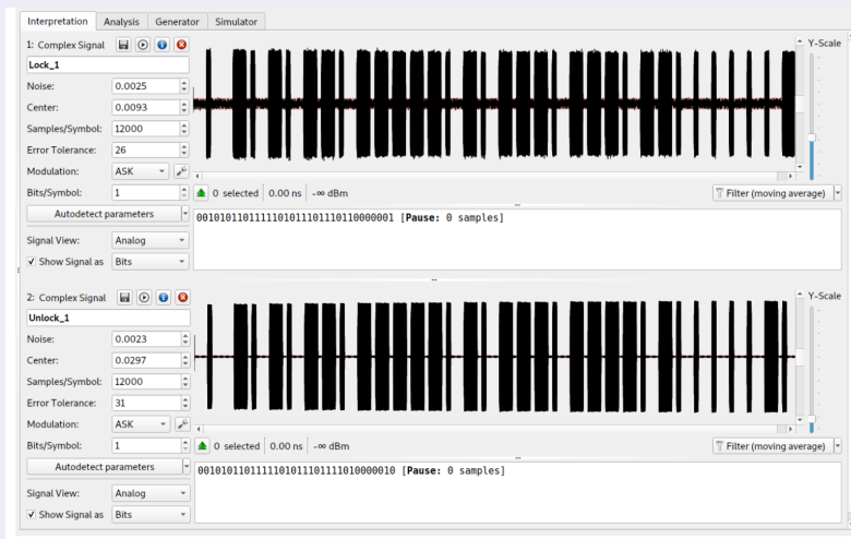
Figure 36. Top signal is lock, bottom signal is unlock. Here we don't know what they are yet but there is some sort of unique binary pattern being produced on the button clicks.
