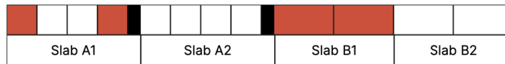
Figure 123. The buddy allocator allocates a slab of objects for the slab allocator to use. Here we have allocated two blocks each for objects of size A and B. Then the slab allocator manages the slabs, minimizing internal fragmentation
