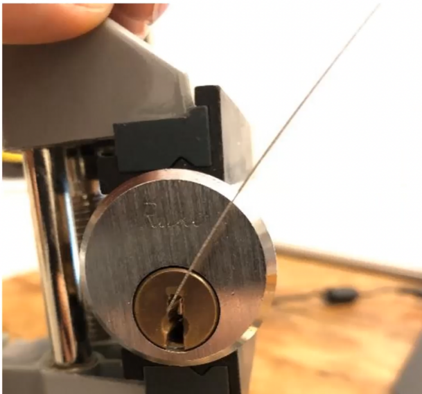
Figure 77. Picking a lock: first, place some tension on the lock
