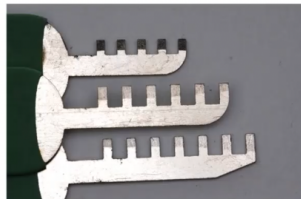
Figure 82. Some locks you can just push all the way up and unlock. Kind of like a buffer overflow. Solutions to this have been created i.e. having a canary pin of sorts which when overlifted jams the lock until the correct key is inserted. Or some other locks where if the wrong key is it shoots you.
